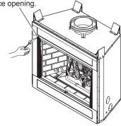
Figure 12 - Checking for Spillage
